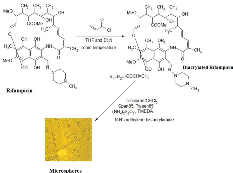
**FIGURE 1.** Schematic illustration of microspheres rifampicin based preparation. [Color figure can be viewed in the online issue, which is available at [wileyonlinelibrary.com](http://wileyonlinelibrary.com).]
